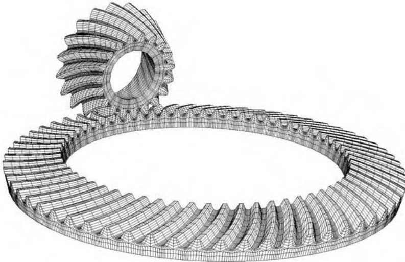
Figure 9.5.3: Finite element model of a whole spiral bevel gear drive.
