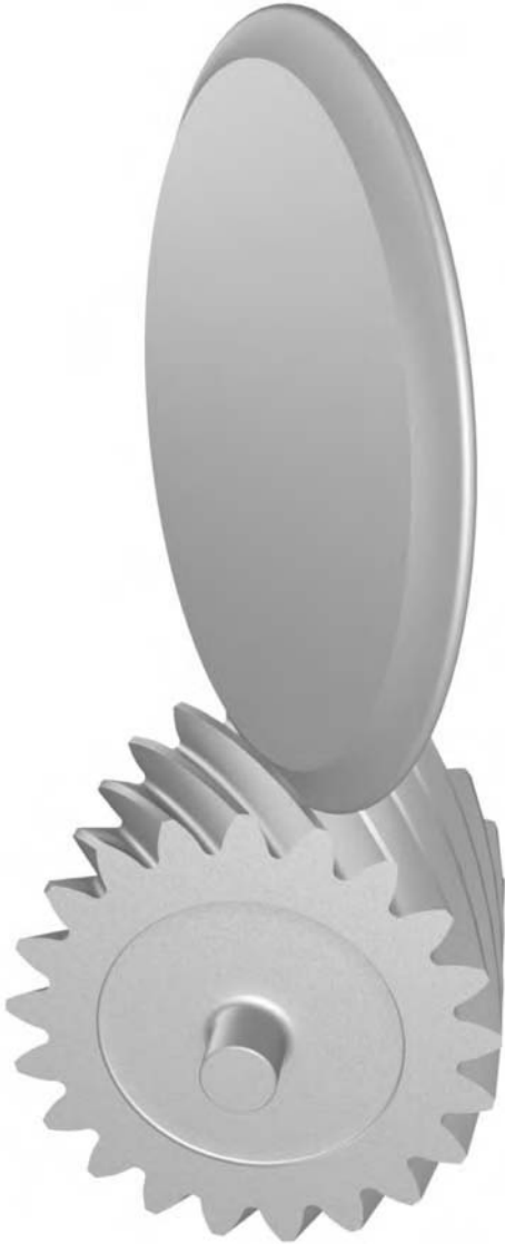
Figure 15.5.1: Generation of pinion by grinding disk.
