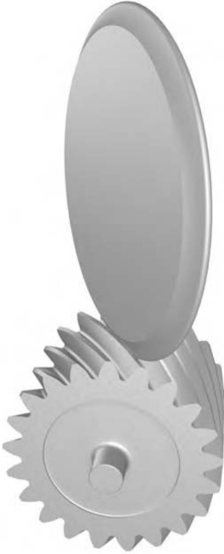
Figure 17.6.1: Generation of pinion by disk.
