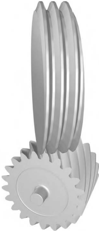
Figure 15.6.1: Generation of pinion by grinding worm.
